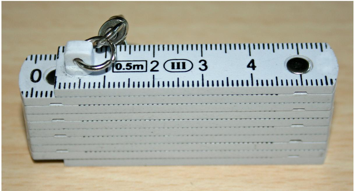
Figure 1 Example of the 0.5 m x 13 mm folding ruler
